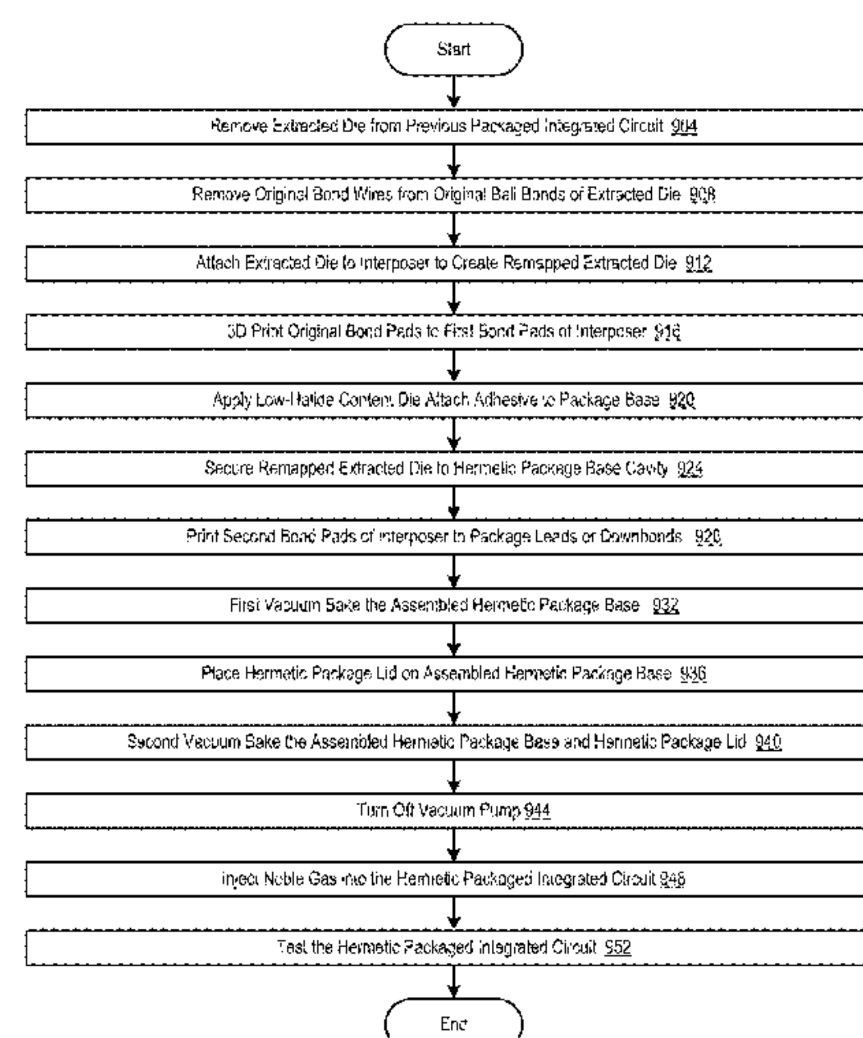
Assembly Method for Hermetic Packaged Integrated Circuit
